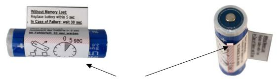
Under the label of the battery is now a flat pin. This pin prevents that the lithium battery in the mounting plate can shift. The battery can not move any more, caused from a shock or push during a transportation for example. The contacts can not be interrupted.
